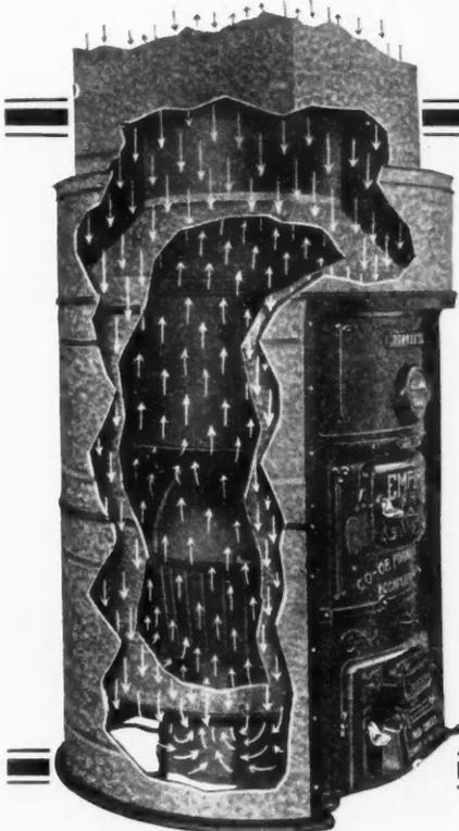
Sectional View, showing Double Casings and Circulation of Air
