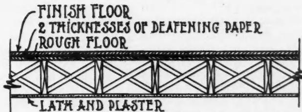
Fig. A. Ordinary Construction Complained of as Not Soundproof.
