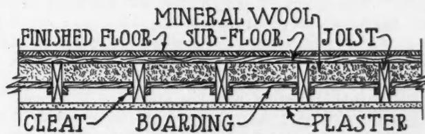
Fig. D. Remedy by Packing with Mineral Wool.
