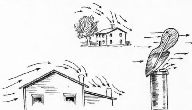
This illustration shows effect of wind currents on flues that do not extend higher than ridge of roof.
