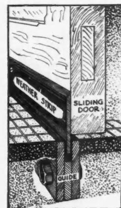
End View of "Schoulers" Patent Weather Tight Door Sill
