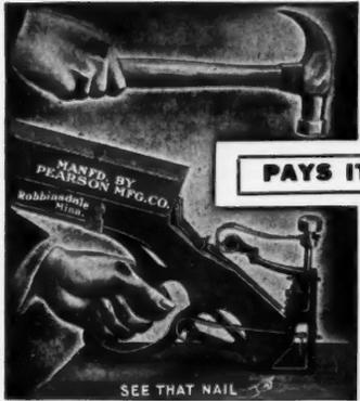
Works well on any pitch roof. Gloves or mittens can be worn and nails driven faster than by the old way. Throw nails in by the handful—holds about 600 nails—start nailing. Nails can be driven through tin or quite heavy sheet iron.
