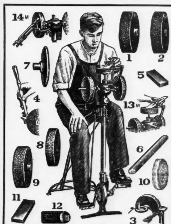
FOURTEEN MACHINES IN ONE. 1—Fine Dimo-Grit Wheel. 2—Coarse Dimo-Grit Wheel. 3—Universal tool rest. 4—Chisel and plane bit guide. 5—Dimo-Grit razor hone. 6—Dimo-Grit scythe stone. 7—Dimo-Grit saw gummer. 8—Felt polishing wheel. 9—Medium Dimo-Grit Wheel. 10—Cloth Buffing wheel. 11—Dimo-Grit oil stone. 12—Dimo-Grit pocket hone. 13M—Plane bit honing attachment. 14M—Twist drill sharpening attachment.
