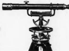
A reliable instrument for simple levelling and laying off horizontal and vertical angles. Can be handled speedily and easily.
