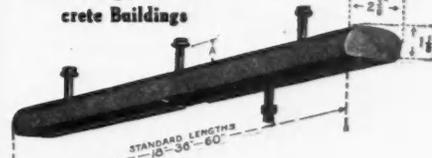
Trus-Con Pressed Steel Inserts are imbedded in the concrete during construction, saving expensive drilling after completion of the work. The long slots allow a wide variation in position. Special washers prevent bolts from turning in the slots. Write for details and prices.
