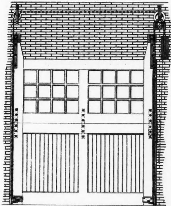
Standard Wood Cross Horizontal Folding Door. Paneled in Upper Half With Glass. This Door Takes up no Valuable Space When Either Opened or Closed
