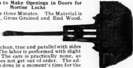
The job is clean, true and parallel with sides of door. The labor is performed with slight exertion. The care is practically none, as the tool does not get out of order. The adjustment is done in a moment's time for the different sizes. The cutters are five in number and cover locks from  $\frac{1}{2}$  inch to  $1\frac{1}{4}$  inches thick. Thin doors are handled as easily as thick doors.
