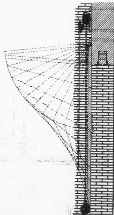
Diagram Showing Different Positions Formed by Door in Opening and Closing
