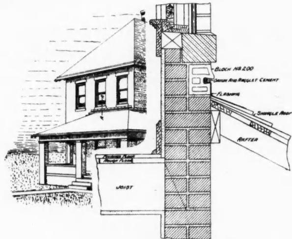
SECTION AT A-A SHOWING RAGGLE BLOCK USED TO RECEIVE FLASHING FOR PORCH ROOF
