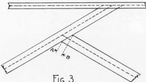
FIG. 3. Intersection When Main Roof is Steeper than Gable
