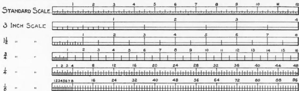
Scales (Slightly Reduced) as Used by Architects in Making Scale Drawings
