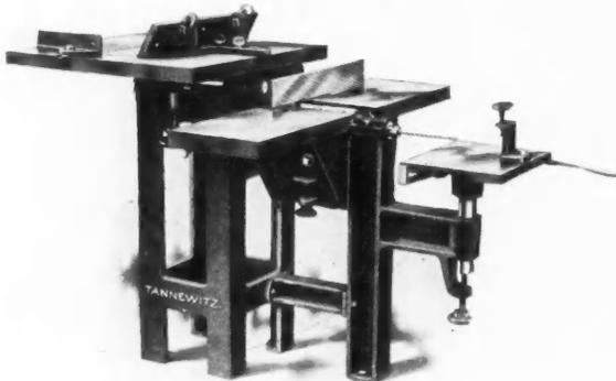
tinct machines permitting three men to work at one and the same time. It is strongly built, being made entirely of cast iron (no wood or angle frame work being used). It is com-
