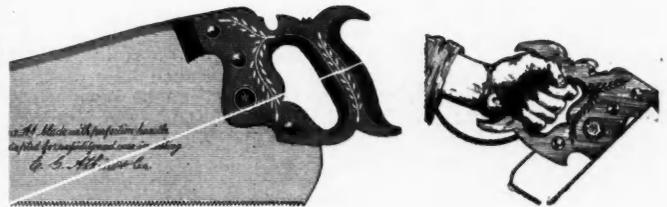
Fig. 1. New Style Handle, Showing Direct Application of Effort to Cutting Edge and Natural Position of Wrist While Using
