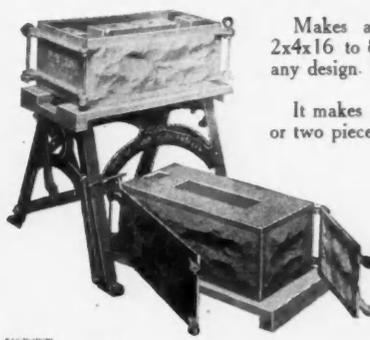
Makes any size block from 2x4x16 to 8x12x20 inches, with any design.
