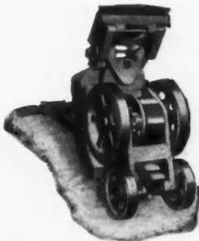
In position for sharpening scraper blade.
