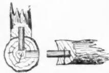
FIG. 2. JOINTS FOR SEAT RAILS TO POSTS
