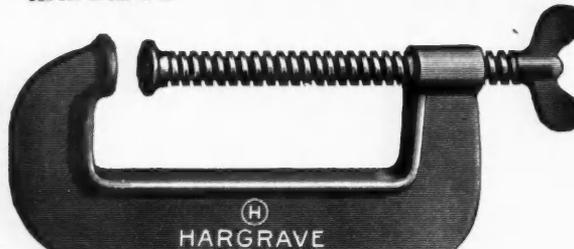
This clamp is thoroughly made of the best refined malleable iron, and is provided with a button tip. It has a very deep, square thread in both the screw and frame, and is in every way the strongest and best clamp in the market. Each size is numbered by inches the thickness of the work it will take in.
