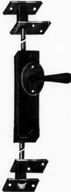
The bolt lies in a groove and is covered with an astragal, attached to the meeting rail of the door or window containing the bolt.
