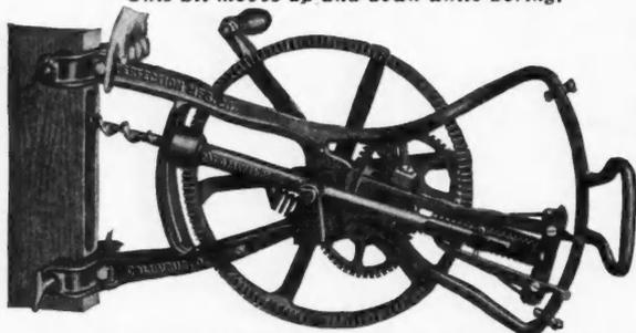
For Door Locks, Sash, Sash Pullies, Screen Frames and Cabinet work. Instantly changed with screw driver, from round hole to ANY size mortise up to 6 1/2". Finished perfect, WITHOUT THE USE OF BRACE OR CHISEL. Made of Malleable. Automatic and ball bearing.
