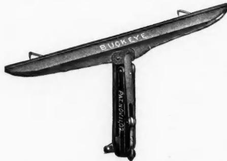
compact form for the tool chest and can be attached or detached to bench without screwing or clamping by means of folding hooks which are driven into the bench.
