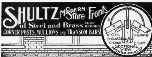
**Handsome, Strongest and Most Practical Bar on the Market. Long Life—nothing to rot out. Glass Bedded on Spanish Cork, preventing cracking or Crushing of glass. No putty, yet ABSOLUTELY WATER AND DUST PROOF.**
