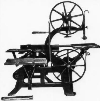
Universal Wood Worker, fitted out with Band Saw, Mortising Attachment, Shaper and Jointer.
