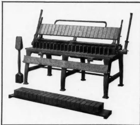
Is the fastest Hand Brick Machine on the Market; will make plain, veneered and ornamental face and shape; all perfect, smooth brick, true to size and design. Send for catalogue giving complete line of Mixers and Brick Machines.
