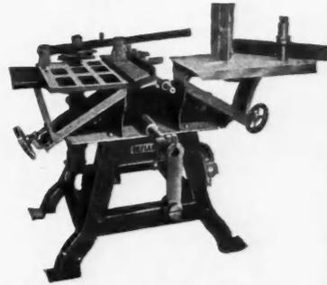
Universal Wood Worker, fitted out with the Single End Tenoning Attachment, with traveling table and hold down lever.
