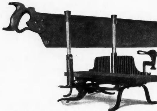
The second cut shows the saw raised to full height so the operator may use both hands in placing stock to be cut. When ready to use the saw all that is necessary is to take hold of the handle of the saw or give the saw guides a light tap on the top and the saw will drop into position ready for use.
