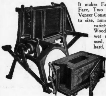
It makes Face Down, Side Face, Two Piece Wall and Veneer Construction. No limit to size, number of shapes or variety of designs. Wood pallets. A very wet mixture can be used, which makes hard, dense and non-absorbent blocks. Absolutely no loss from chipped edges or cracked blocks.
