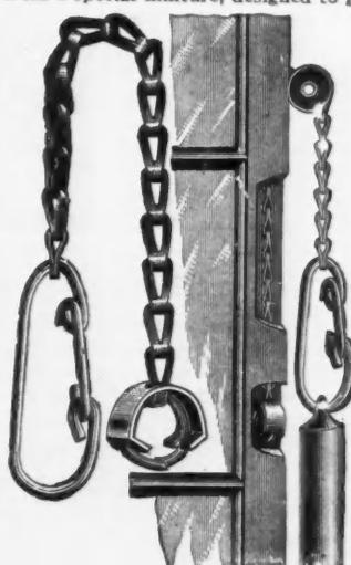
The formation of the link, being flattened at the bend, prevents friction in running over wheel of pulley, adds to the strength and prolongs the life of the chain.
