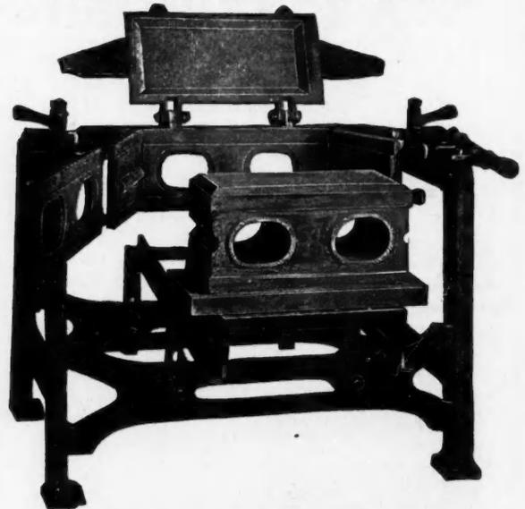
The **SUPERIOR** makes the stone with the face down or in the bottom of the flask, which permits of the use of fine rich material for the face and coarser, cheaper material for the main body of the block.
