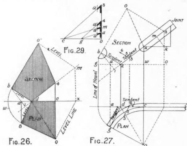
the plan in Figs. 21 and 22, and on  $s$  as a center describe a circle having a diameter equal to the width of the straight rail. This determines the width of the mold at this point.
