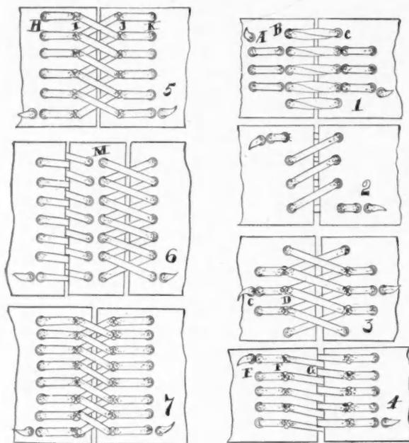
end. Then we repeat the sewing of the lace end on this opposite side, and return across. The operation is simply repeated until the entire distance across the leather belting is covered. The result is that quite a powerful union has been produced, and yet there is much flexibility at the common center, for the joint can be bent very readily and easily. This type of lacing is calculated for surface on woodworking machinery where there are wheels of small diameter operated at high speed.
