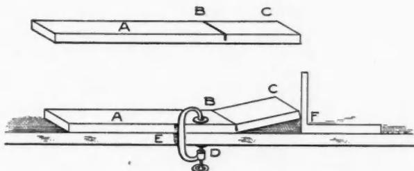
say a writer for any journal should be careful how he says can't or can't be done. Saw kerfing is the simplest thing the mill man has to deal with, by the method I show with two simple illustrations a piece of wood may be bent to any radius no matter how thick or thin the material may be, or how thick or thin the saw may be.
