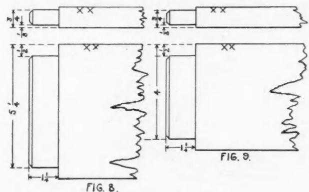
one-half inches and square a light, sharp pencil line across the four legs at this point. Again, measure three and one-half inches from this line and square a line across. Measure from the line last drawn thirteen and one-half inches and mark, then four and three-fourths inches. There should remain between the line last drawn and the end of the leg seven and three-quarter inches. These marks should be on the sides of the legs which have no XX marks on them,
