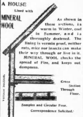
As shown in these sections, is warm in Winter, cool in Summer, and is thoroughly deaired. The lining is vermin proof, neither rats, mice nor insects can make their way through or live in it. MINERAL WOOL checks the spread of Fire, and keeps out dampness.
