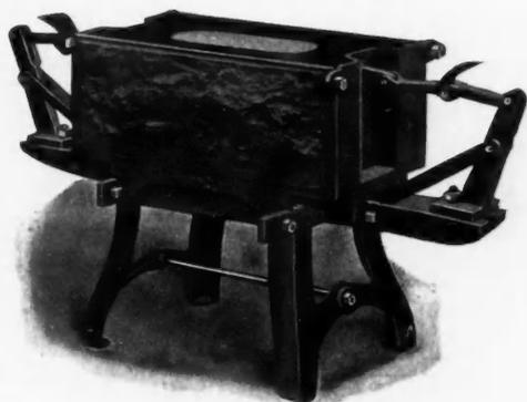
STATIONARY CORE—CLOSED FOR FILLING
