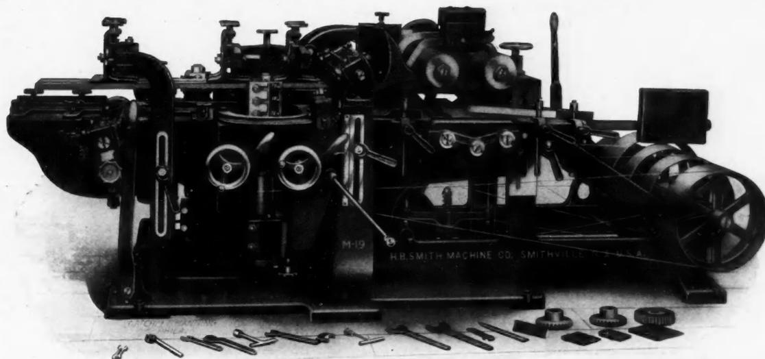
NO. 105-A, EXTRA HEAVY 12-INCH OUTSIDE MOULDING MACHINE TO WORK FOUR SIDES
