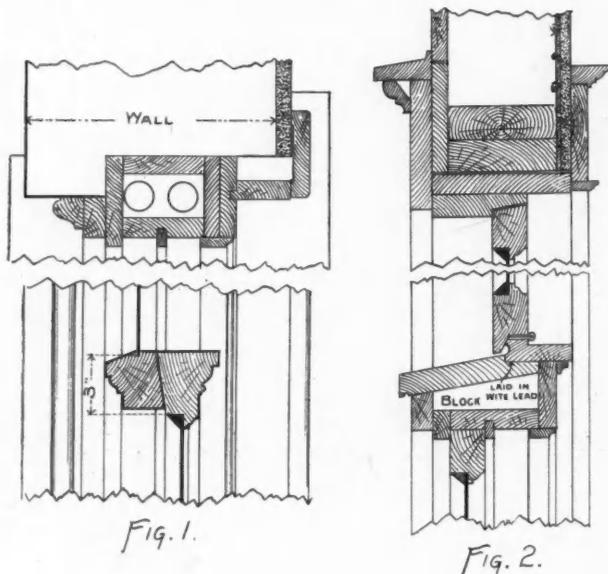
lowered at will, leaving no open joints for the wind and rain to get in when closed. It is well nigh impossible to construct a transom when hung with butts and have it weather-proof. In such cases the most satisfactory way we have found is to hang the sash at the bottom similar to that shown in Fig. 2. This makes a fairly tight job and is simple in construction.
