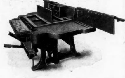
**No. 9.** Open. Set for 1-10x32 in. straight and 1-10x32 in. corner. Rock face inside angle, plain division. Use rock face division and rock face end to rock face outside angle.
