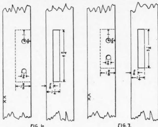
leg so that when the XX marks are placed outward with reference to the framework, the best surfaces shall face forward and outward. The same precaution should be taken in marking the faces of the rails.
