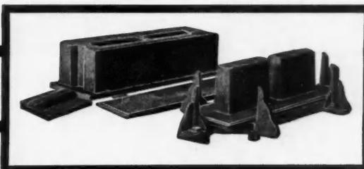
The Clipper Block Machines are simple, durable, light, strong, accurate, and will produce a great variety of shapes and sizes in hollow blocks, veneering blocks, chimney blocks, pier blocks, circular blocks.
