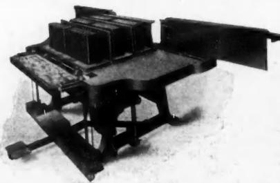
**No. 2.** Front and end view. Set to mould  $\frac{3}{4}$ x32 inches. Cores raised, pallets and divisions in position. Mould box ready to close. Name stamp on one division.
