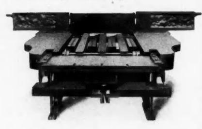
**No. 12.** Open. Cores withdrawn. Divisions removed. 24 inch rock face doors shown. The No. 4 Chicago is the only perfect adjustable machine.
