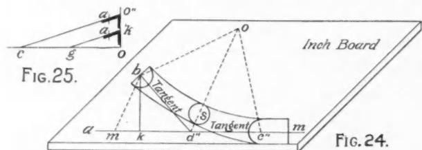
the board equal to half the width of the rail and transfer to it the points  $mkd''c''$  either from the pitch line in Fig. 21 or in Fig. 22.
