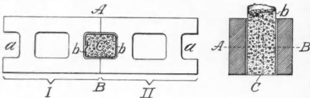
The vertical recess (a) of adjacent ends form a comparatively large vertical chamber. A loose roll (C) of tarred paste-board, felt, asphaltic felt or other suitable material is placed in each said chamber.
