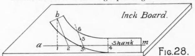
the Figs. 21 and 22, and  $ok$  equal to  $ak$  in the same figures; connect  $kg$ . The bevel will be at  $k$ .
