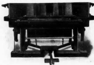
**No. 11.** Open. Cores raised. Pallets in position. Center division not in. Has 2 sides of any design wanted.
