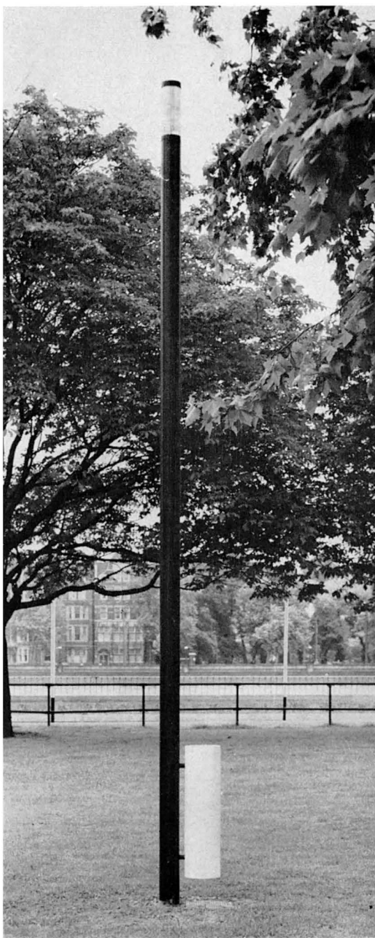
4. Commended entry designed by Richard Stevens, Peter Dodd and John Barnes. 15' steel column; made by Atlas Lighting Ltd., London.
