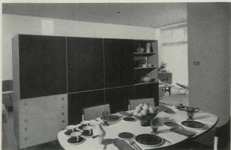
Cabinet was designed specially for this house, and built of ash plywood with black plastic panels bonded to hardboard.
