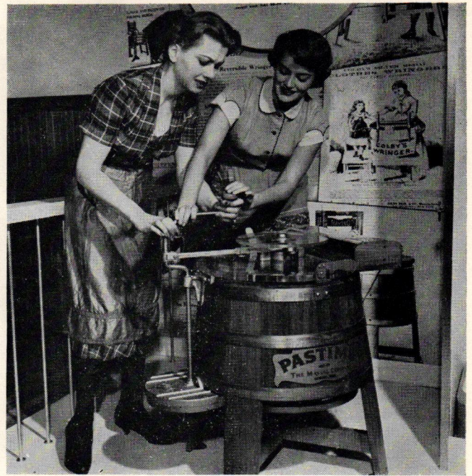
One of the first washing machines featured an outside crank, which rotated a contraption that turned clothes through the water, scrubbing them against the sides and bottom of a cypress tub.
