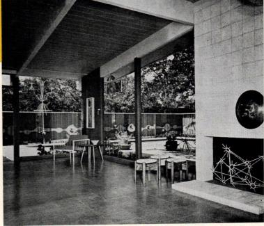
imagine possible in cold weather. Insulating glass consists of two or more panes of glass, with a hermetically-sealed dead air space between.
