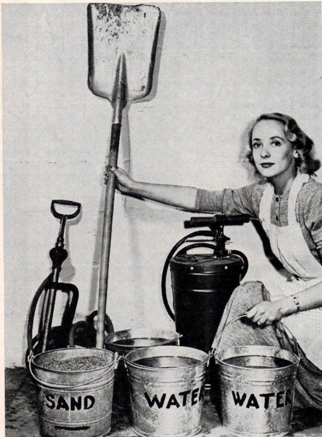
Minimum fire-fighting equipment which will be essential in any bombing attack: a stirrup pump with hose, several buckets of sand and water and a shovel. Each member of the family should learn to operate the hand pump.
