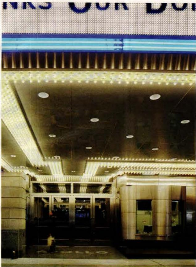
The original flashing, chasing pattern of the bulbs has been reinstated on the marquee's underside: four on, one off, enticing audiences inside. Zinc Moderne letters are inlaid into new terrazzo flooring alongside a rounded steel ticket booth at ADA-compliant height and replicated limestone-and-granite pilaster bases. *Photo: Elliott Kaufman*
