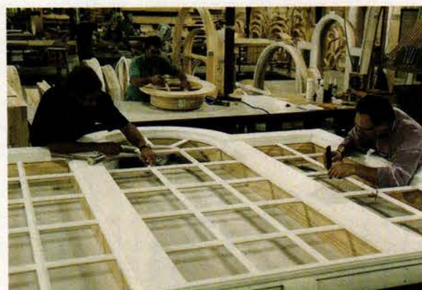
Custom windows in non-standard sizes and shapes, such as this divided-lite model, are fabricated by Parrett Windows . Write in No. 3003
