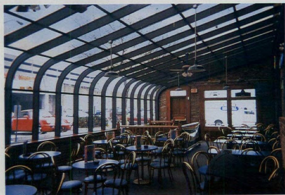
Seen from within, the custom-designed solarium features 1-in. insulated bronze glazing throughout, and a bronze aluminum, duracron/polycron finish. (Photos: Commercial Sunroom Products Division of Patio Enclosures, Inc.)
