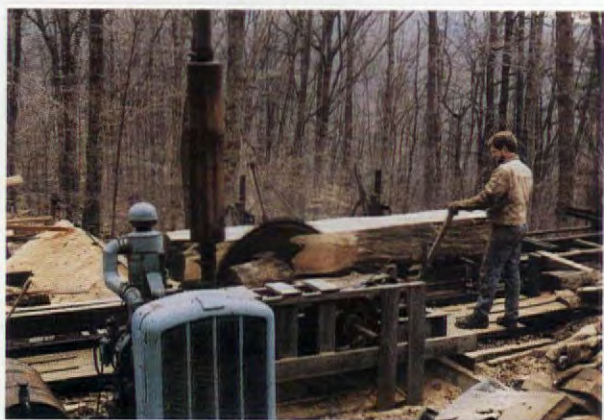
Dean Fitzgerald cuts a heavy beam with his 50-year-old Frick Mill. Much of the timber taken from the bridge during its restoration was remilled and reused.
