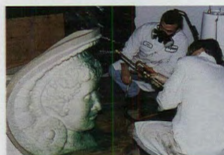
Liquid Polygel Mold Rubber is sprayed onto a GFRG ornament by technicians at POLYTEK DEVELOPMENT CORP. The product is ideal for the reproduction of ornament and sculpture. Write in No. 6560
