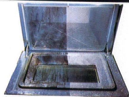
Half Perma-Clean, half regular porcelain oven after 150 hrs. heavy usage.
