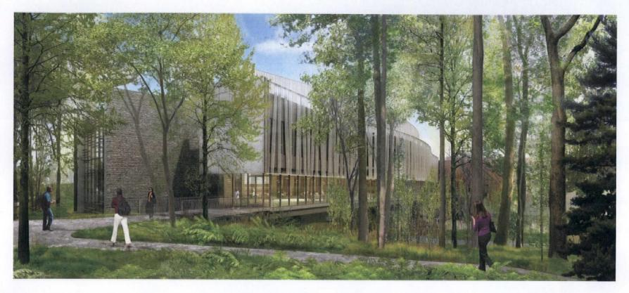
overhang of the upper level recesses the glazing, limiting reflections of sky and narrowing the angle from which birds can see habitat reflections. On the upper levels, vertical shading fins similarly reduce reflections and birds' angle of view to the glass.
