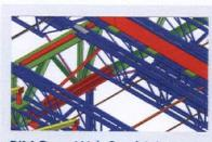
BIM Open Web Steel Joist Design
