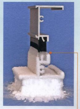
Extreme cold temperatures of -100°C (-148°F) will not transfer through an aluminum frame with a modern pour and debridge thermal barrier ( and neither will high temperatures in very hot environments)
