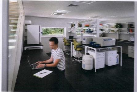
WARREN WOODS Architects from GO Logic designed a field station (above) for the University of Chicago, in Berrien County, Michigan, so that its laboratory (left) serves as the heat engine for the rest of the building. The excess heat produced by the research equipment is captured and ducted to the other rooms.
