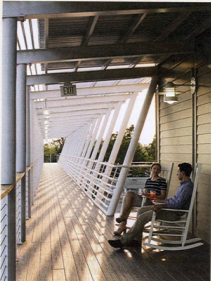
Porch overhangs intercept train noise and protect the interior from solar thermal gain.
