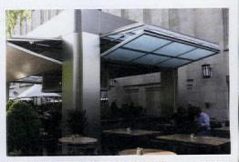
HYDRAU-LIFT™ BI-FOLD DOORS SNAP 63 The Hydrau-Lift™ automated bi-fold doors quickly open your restaurant, hotel, bar patio, pool area, sky boxes and even large interior spaces. The special lift system forms a tight weather and sound seal around the door.
