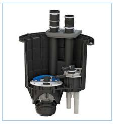
A cutaway of the **new Sanipit 24GR retrofit pump kit** shows its interior components, including (on the left) the grinder pump with a powerful 1-horsepower motor and stainless-steel grinder blade and a fail-proof, air-pressure switch system (right) with triple redundancy.
