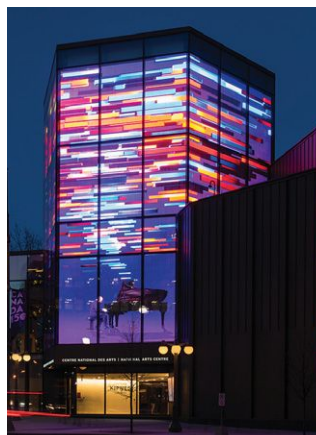
A TRANSPARENT LED SCREEN HUNG LIKE A SCRIM INSIDE THE ENTRY TOWER'S GLAZING PUBLICLY SHOWCASES ARTISTS AND THE PRODUCTIONS INSIDE.
