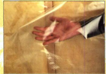
Made from an advanced material that changes its permeability with the ambient humidity condition, MemBrain™ Smart Vapor Retarder from CertainTeed Insulation allows closed building envelope systems to increase their drying potential with seasonal climatic changes—reducing moisture by as much as 80%.
