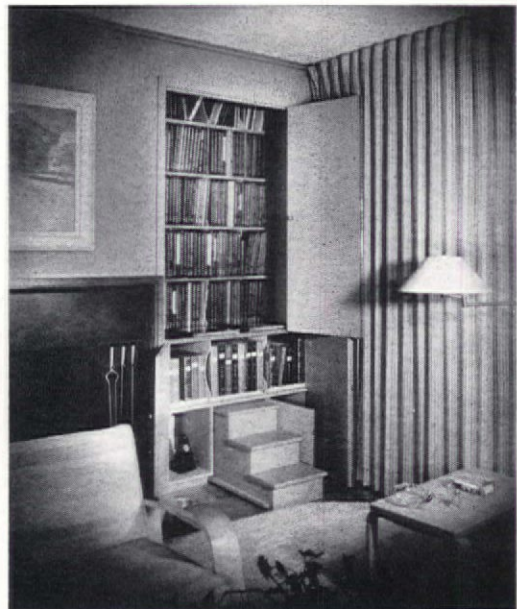
"That's for me" . . . we can hear the chorus certain to greet this idea. Hide-away steps for short stretchers glide out on their own guides and rollers. They are locked safely in place by a latch on concealing door
