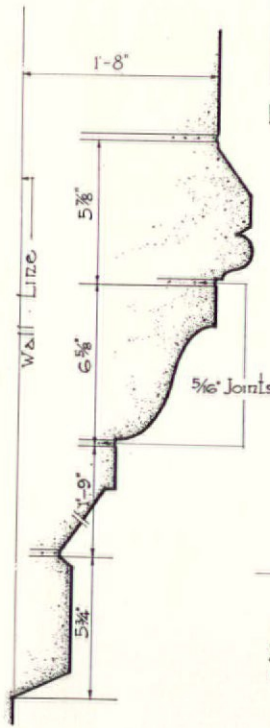
PROFILE OF STONE CORBEL ON C of BAY Scale: 1 1/2" = 1'-0"
