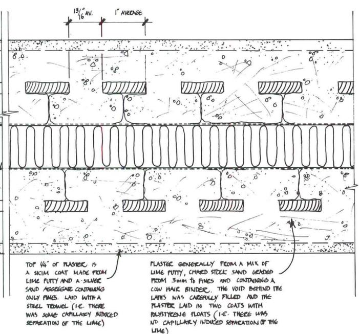
HORIZONTAL AND VERTICAL SECTIONS THROUGH LIME PLASTER WALL
