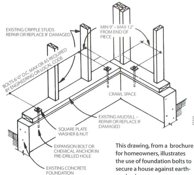
This drawing, from a brochure for homeowners, illustrates the use of foundation bolts to secure a house against earthquake damage.
