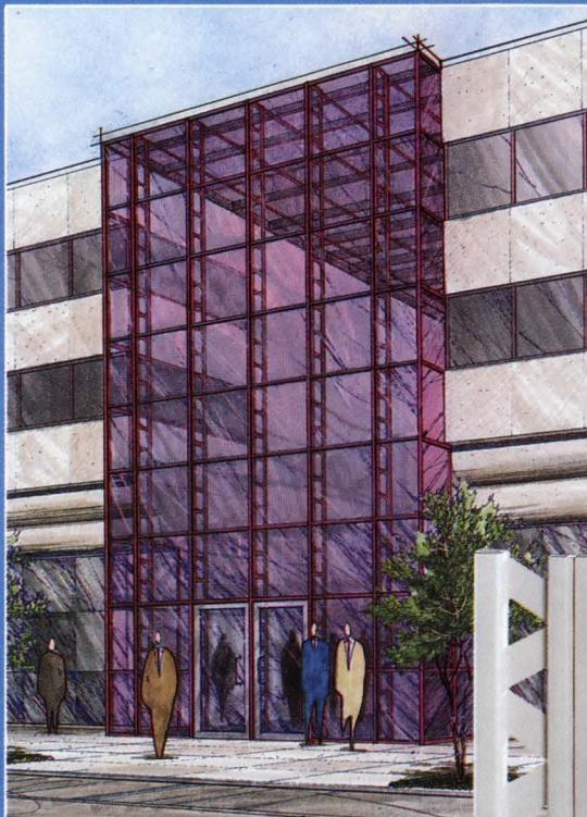
But while the design options offer flexibility, the integrity of the structure remains inflexible. A thermal break, and the flexibility of either  $\frac{1}{4}$ " or 1" glass attest to Trusswall being ready and willing to take on nature's harshest elements.
