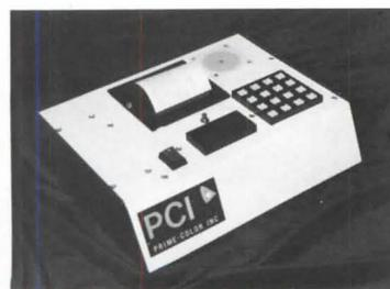
**Prime-Color:** Illumination quality meter is a sophisticated, handheld, computer-operated light-measuring device.
