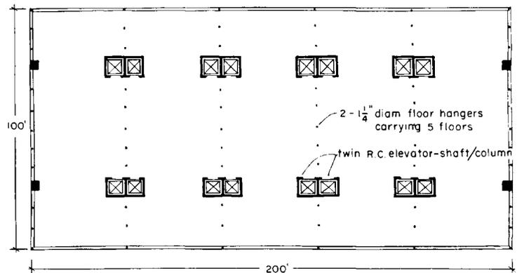
area of each story is totally unobstructed and at the same time a continuous free span can be provided along the entire perimeter of the building. Extending further this examination of utilizing suspenarch structures in conjunction with elevator-shaft/columns, a 30-story reinforced-concrete structure was next investigated.
