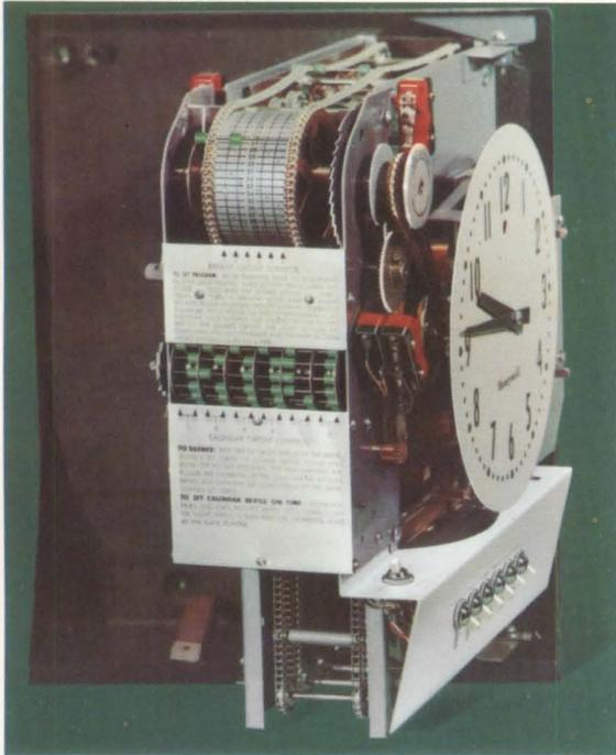
**Easy-to-set signal drum.** Honeywell's Clockmaster eliminates fuss and bother from program setting. Just turn signal drum to time, slip steel pin through chain links and slide on one of the reusable plastic rollers. To change signal, roller can be shifted without affecting any other part of the program. Special round pin-in-square-hole construction holds each signal roller firmly in place.
