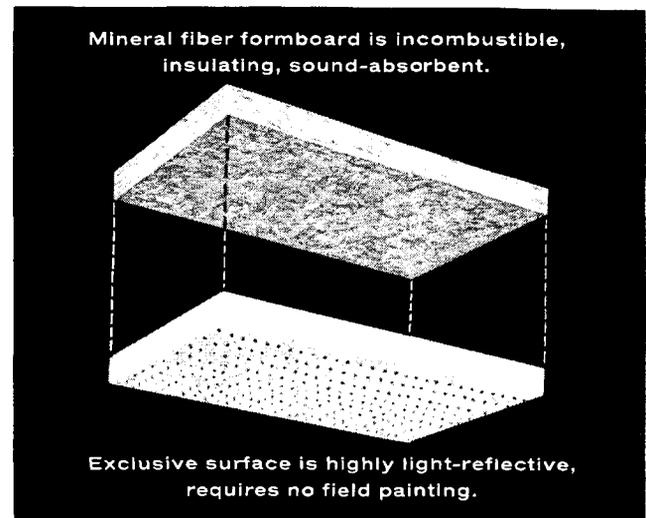
The durable, light-reflective surface that covers the underside, ends and sides of PYROTONE is manufactured right into this mineral fiber formboard. This bright surface retains its beauty and simple elegance, assures easy maintenance through the years.
