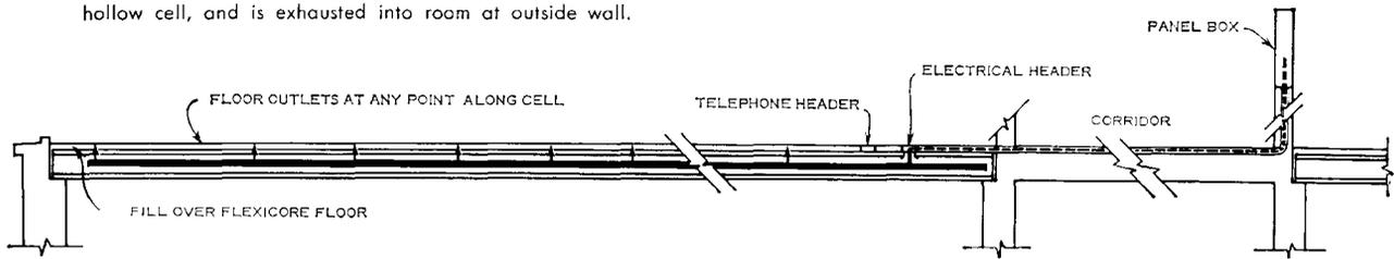
Section BB. Electrical wiring runs from panel box, through header, then through Flexicore hollow cell to floor outlet. Similar system is provided for telephone.
