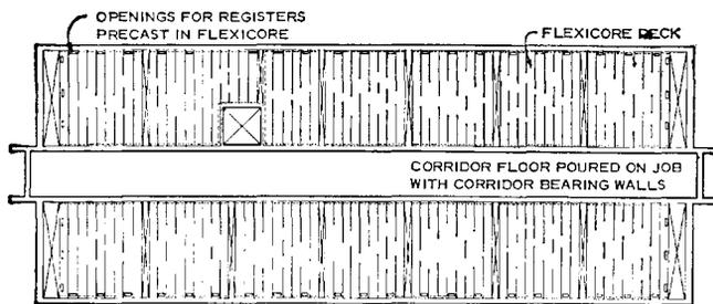
First Floor Framing. Corridor floor was cast in place with corridor bearing walls. Flexicore clear-spans from corridor walls to outside walls.
