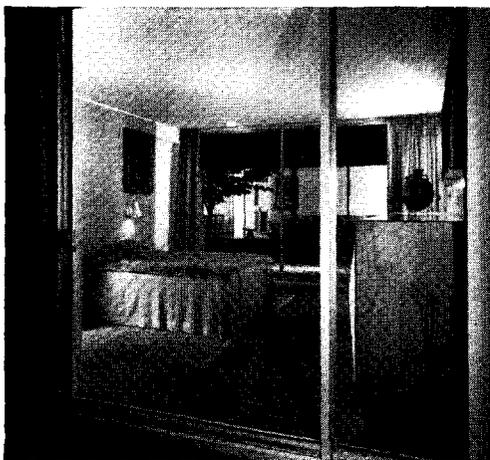
*In this Sert bedroom, as in other rooms, return air for the Lennox heating-air conditioning system is taken high in the room, with 80% of grille work concealed behind a cove moulding.*
