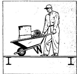
**STRENGTH.** Angular pattern with wide rib openings provides strong section properties. Granco Deck supports wheelbarrows, welding machines, etc., without bending or buckling.
