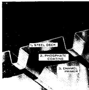
**TOUGH FINISH.** Rust-preventive enamel is "flow coated" over steel, baked on at 350° F. for 20 minutes. Flint-hard finish prevents corrosion, resists abrasion from field handling.
