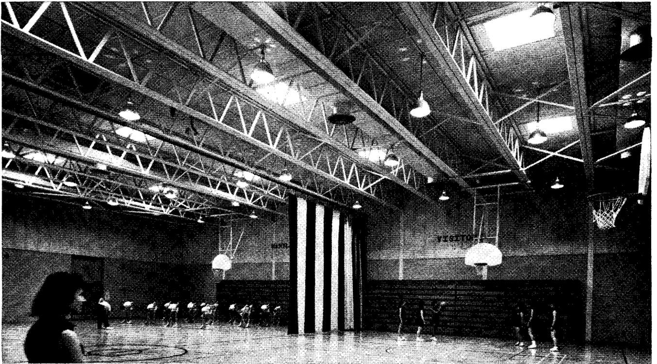
**GYMNASIUM** incorporates both Tectum roof deck and sidewall panels for maximum insulating and acoustical value. Roof deck is 2½" thick; sidewall panels are 2" thick with neat beveled edges and tongue and groove joints. *Four walls and a ceiling for effective sound control* in an area where noise can be a problem during study periods.
