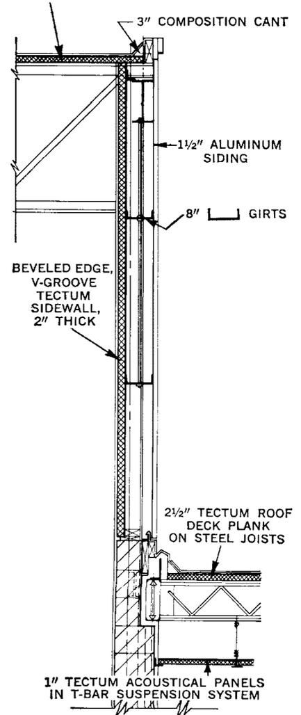
Detail of gymnasium wall showing Tectum sidewall, roof deck, and corridor acoustical ceiling.
