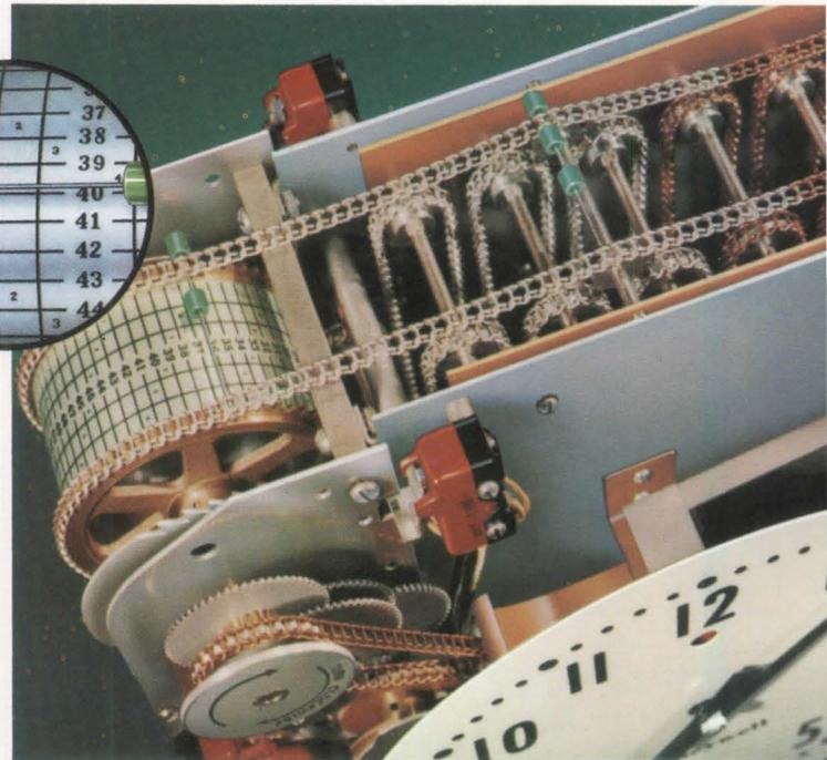
**Easy-to-read numbers: Link chain ruggedness.** Numbers on the signal drum are large, easy to read, and never confuse the program setter. Two precision link chains, color-coded for day-night identification, guide the entire program whether it includes three circuits or six. Chains are rated at twenty times load for insurance against breakage. Chains run continuously over idler gears. No piling at bottom of cabinet.
