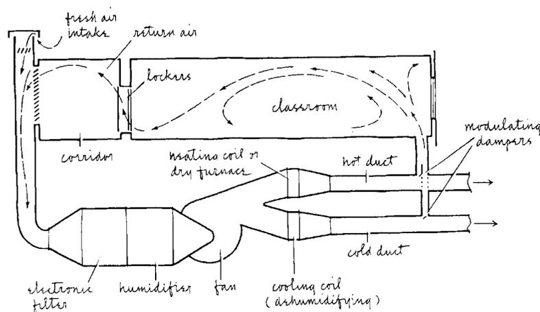
Diagram of air-heating system.
