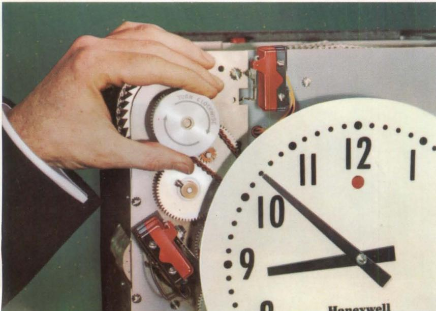
**Dial-it clockwise program unit.** Master time and master signal units are positively linked together. No chance for them to get out of step. When a program is set, the time setting knob is turned. As the clock hands reach the desired time, the program drum turns, too. In the same way, if power is interrupted, programmer runs on spring power with the master clock. When power is restored, signals again are right on schedule.
