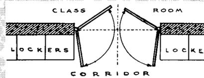
**2** RIXSON DUO-CHECK operating Double Classroom Doors swinging both ways. With half the wall thickness and locker depth adding up to 23", these doors when open 90° will extend only 5" into the corridor. Small 2'4" doors on Duo-checks panic proof for small children.
