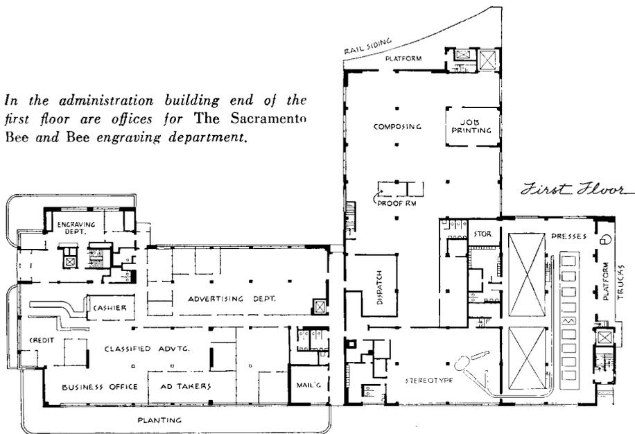
Rolls of newsprint arrive on the rail-freight siding and are taken to basement storage by elevator; ink tanks are filled through curb boxes on 21st Street.
