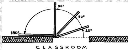
**1** RIXSON UNI-CHECK with 4 points of hold-open. A 180° hold-open built into the Uni-check plus 3 additional hold-open points in the RIXSON No. 37 Holder . . . allows teacher to set door where desired. A slight push releases hold-open. The ideal classroom door control.
