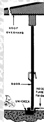
**RIXSON** heavy duty closers (single and double acting) have controlled the action of school entrance doors for over 40 years; lighter double and single acting RIXSON concealed, floor type closers are being used in different applications for school classroom doors, office doors, toilet room doors as well as doors leading off the corridor into stair wells. Shown above are four interesting applications . . . further details available.
