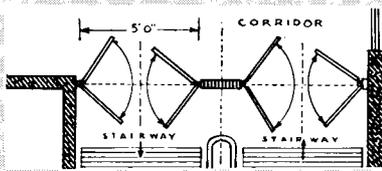
**3** RIXSON No. 30 Double Acting Closers operating doors leading into stair well. This arrangement allows a free traffic flow. Small 2'6" doors easy for small children to open.
