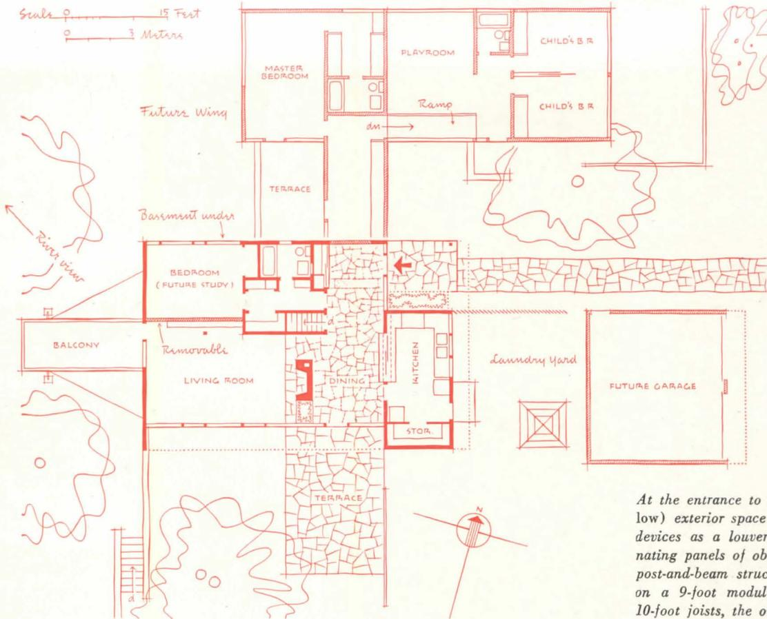
At the entrance to the house (two photos below) exterior space is defined by such various devices as a lowered wood fence and alternating panels of obscure and clear glass. The post-and-beam structural system was laid out on a 9-foot module, allowing direct use of 10-foot joists, the overlapping providing effective tie. Posts are 4 x 4's and beams, 4 x 14's.
