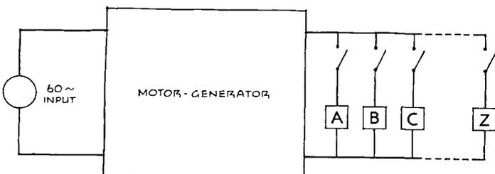
Figure 5—group operation circuit
