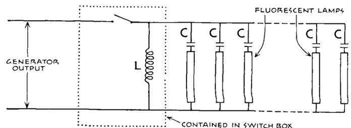
frequency (Figure 4), and the Group Operation Principle is employed. The auxiliary equipment is not designed as a one- or two-lamp ballast, as generally used today, but is arranged for the entire group controlled by a single wall switch. Much of the auxiliary can then be enclosed in an acoustically-treated wall switchbox.
