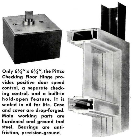
Only 6¼" x 6¼", the Pittco Checking Floor Hinge provides positive door speed control, a separate checking control, and a built-in hold-open feature. It is sealed in oil for life. Case and cover are drop-forged. Main working parts are hardened and ground tool steel. Bearings are anti-friction, precision-ground.
