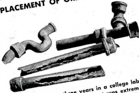
Ordinary iron soil pipe after three years in a college laboratory. Since it was concealed in the ceiling, replacement was extremely costly. The Duriron pipe which replaced it has caused no expense since its installation sixteen years ago.
