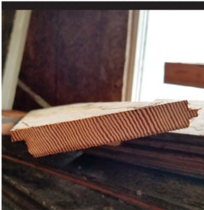
LEFT A sample of the 1" thick vertical-grain Douglas fir that runs throughout the house. The owner was able to use scraps from boards that had to be replaced to make repairs in other locations. BELOW Electrical lines ran under the patch.
