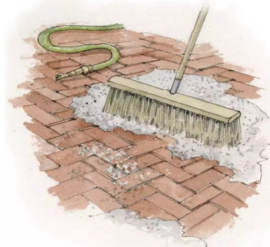
DRY GROUTING WITH STONE DUST
