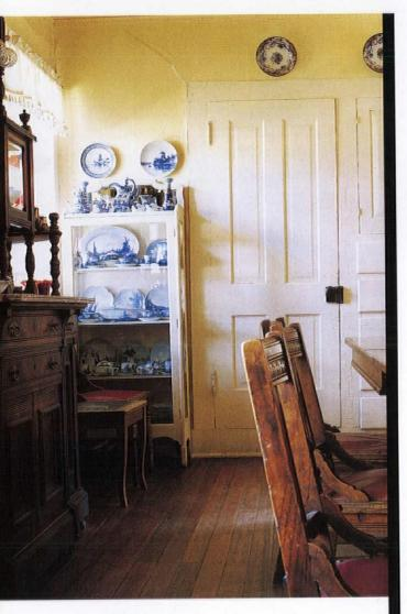
ABOVE A raised panel door that doesn't quite close at the top may be suffering from excess paint buildup, either on the door or on the hinges.
