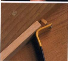
TOP To remove a stile, first remove the pegs that hold it to the tenon on the rail using a pin punch that's smaller than the peg. ABOVE To extract a stubborn wedge that hasn't been glued in place, drill a screw into the wood, then ease the wedge out with a claw hammer. RIGHT To remove the door, first loosen and remove the hinges. Hold the door steady or wedge it underneath to take weight off the hinges.
