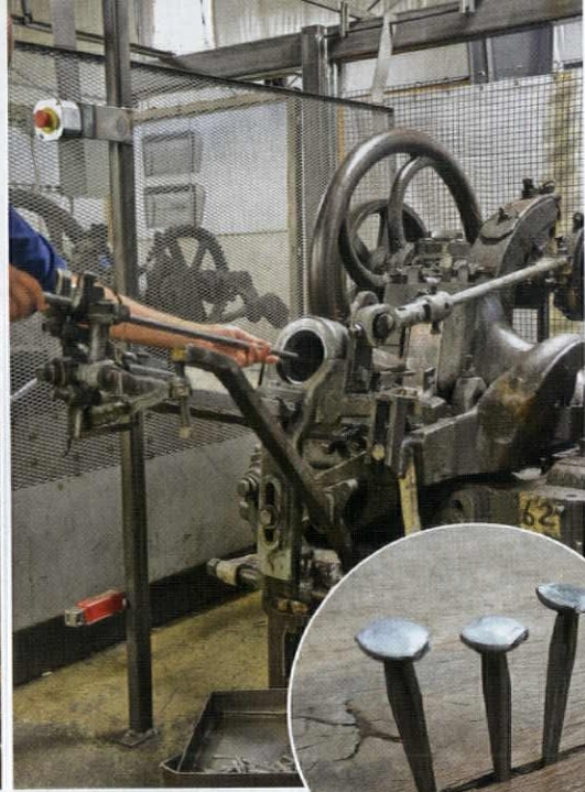
Other nails are made by hand feeding strips into the machine; the tool holder must be turned after every cut.
