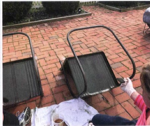
3. Here the homeowner and her friend apply the first coat of Penetrol, a paint additive that adds a soft, sealed finish to metal.
