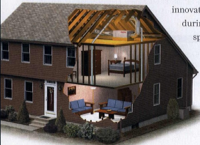
LEFT SpacePak's high-velocity system delivers warm or cool air from an attic unit through flexible, 2" ductwork that snakes between studs in walls.
