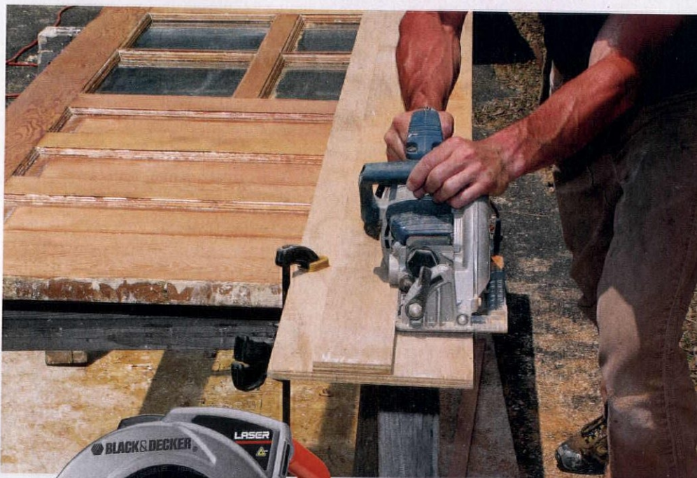
Circular saws, whether worm-drive (above) or sidewinder (left) can team with a shoot-board to make long, accurate cuts, as above.
