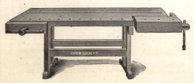
THIS illustration shows our regular Cabinet Makers' Bench. This bench is made entirely of maple. The top is made of  $2\frac{1}{4}$  inch strips glued together to prevent its warping. The working top of the bench measures 78 inches long and 24 inches wide. We also make a smaller size, 66 inches long and 20 inches wide. These dimensions do not include the screws. 34 inches high.
