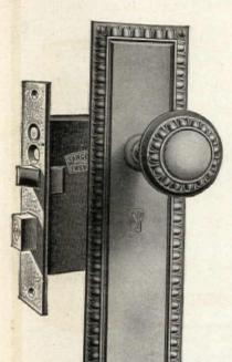
The lock of this front door set has a cast bronze metal front, antique copper finish, 5-16 swivel spindle hub, bronze metal bolts and steel keys. The latch and dead bolt are operated by one key. The knobs and escutcheons are wrought bronze metal, antique copper finish
