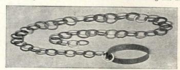
ber of cuts, the condition of the blade was so good that the teeth are clearly defined, even in this greatly reduced illustration. The remarkable flexible property of this blade is shown by its being bent in a complete circle.
