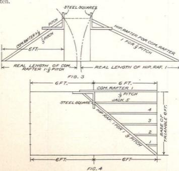
Now, there are few practical facts about the square, which are very useful to know in connection with these problems. For instance, the cut for a quarter pitch is 6x12 for the common rafters. Now, as 12 is to the common rafter, so is 17 to the hip rafter, so
