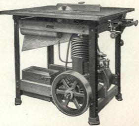
Type "A" with 4 H.P. Gasoline Engine. Weight equipped for work 350 lbs.
