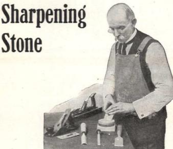
Always free, clean and extra fast cutting-never filled or slick, the round Carborundum Combination Stone is ideal for carpenters' use. Shaped to allow for rotary motion in sharpening chisels, plane bits, etc. For cabinet makers' tools, etc., requiring an extra fine, delicate edge, there is the Carborundum extra hard, extra fine stone.
