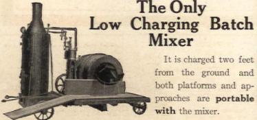
It is charged two feet from the ground and both platforms and approaches are portable with the mixer.
