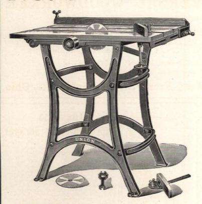
A well built, light power machine, at a low cost, has a wide range for work, will rip stuff up to 31 in. thick, also cut off, miter, and with attachments, bore, edge-mould, groove, dado, etc.
