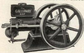
The gasoline engine has done wonders in the building construction field. It has made it possible for the contractor and builder to buy and operate power woodworking machinery and use it that many jobs of millwork formerly turned over to the
