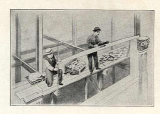
A double spring clamp permits attachment to any ordinary steel square, giving a perfect plumb and level. It can also be fastened to a regular pocket rule, a machinist's steel scale or a strip of wood for leveling larger surfaces.
