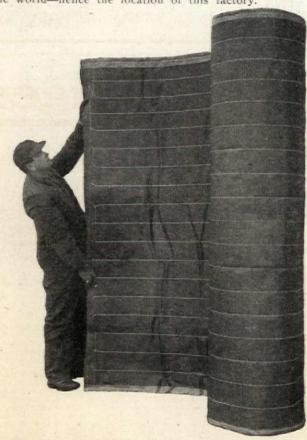
Linofelt (pronounce the "i" as you would in "light") is an insulating quilt made of degummed flax fibre, felted and stitched between two sheets of rosin-sized building paper. By this degumming process, all the vegetables, gum and oils are extracted from the flax straw and thereby all source of decay or disintegration is removed. The reason that a woolen blanket is warmer than a cotton one is because the wool fibre contains more of the tiny air spaces than the softon
