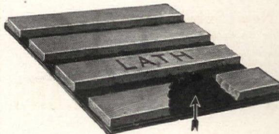
*Shows construction of Bishopric Sheathing. Arrows point to Asphalt Mastic into which laths are imbedded.*
