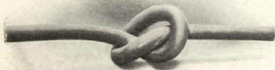
ONE INCH BAR OF VANADIUM STEEL TIED INTO A KNOT COLD. ELASTIC LIMIT 100,000 LBS.
