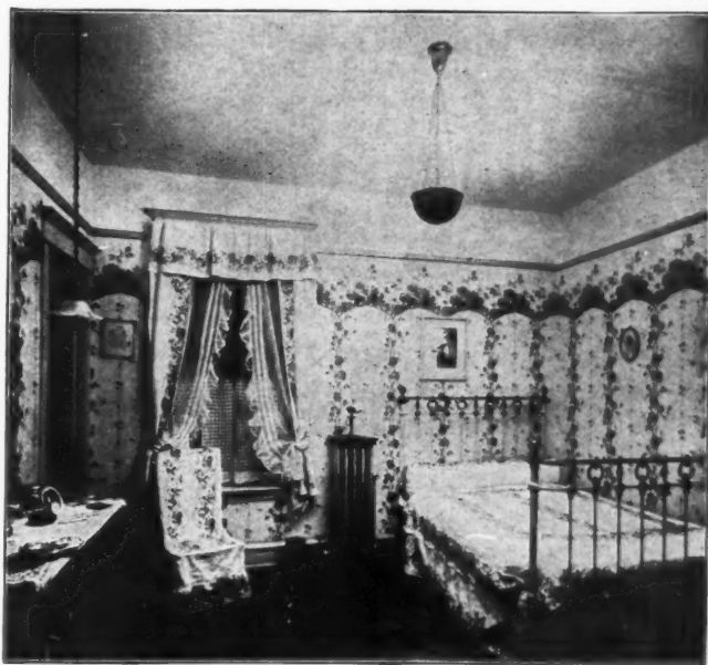
Photograph of this room, 14 feet square, taken by the indirect illumination of a one unit electric fixture containing one 60 watt tungsten lamp. The consumption of current only being equal to that of one 16 candle power carbon filament lamp.
